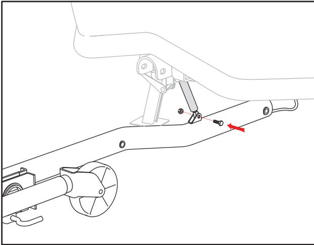
Rotate the tongue into proper orientation and attach the tilt damper end eye to the bracket at shown using the M8 bolt provided.
