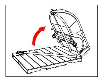
Place the pallet on a flat, level surface. Remove all packaging and carefully rotate the trailer up onto its rear end.
