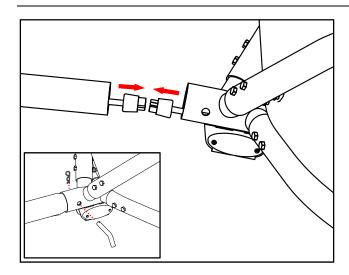
Connect wire harness plugs. Then lift the front end of the trailer body to install the trailer's *Draw Bar* assembly. Insert the *hitch pin* and secure it using the *retaining clip*.
