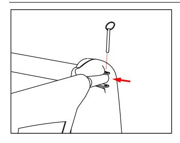
Install *Tailgate*. Attach clips at lower corners. Insert crossbar in brackets and insert *retaining pins*.
