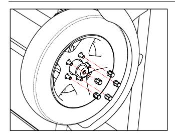
Install *Wheels* and *Lug Nuts*. Partially tighten the *Lug Nuts* and the lower trailer to the ground before completing this operation.
